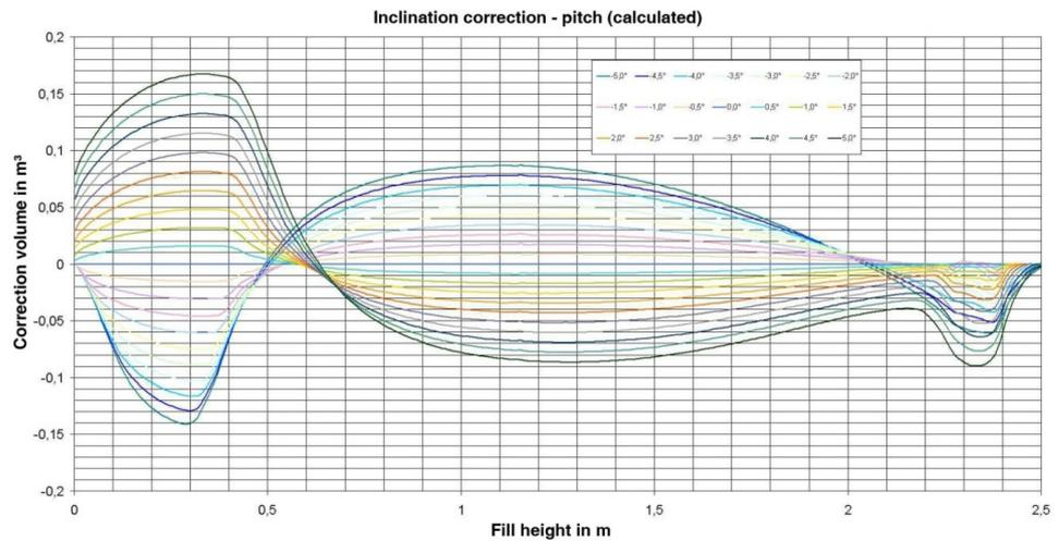
Figure 15: Typical inclination correction curves
