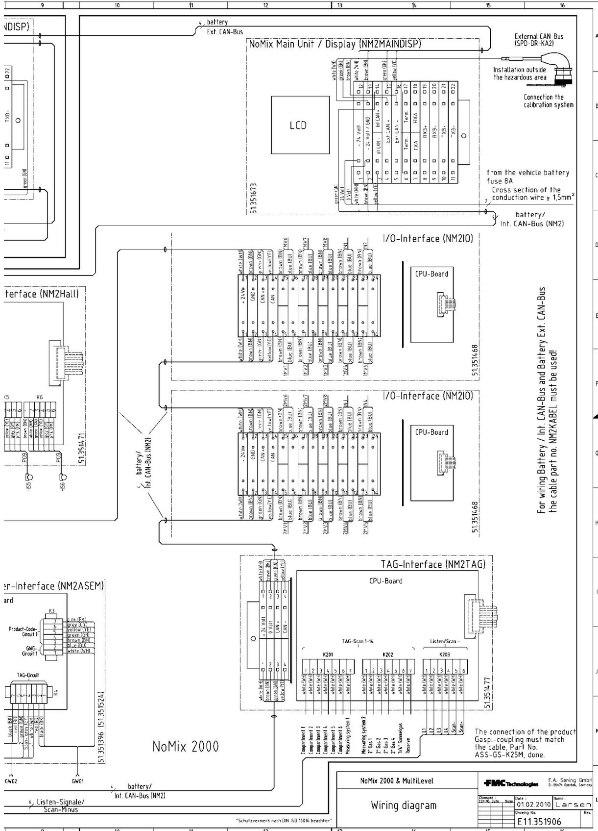
17.1.27. 11.352185 – Overall wiring diagram - MultiLevel – 1 of 2
