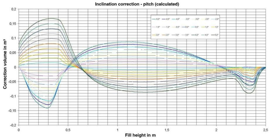
Figure 6: Typical inclination correction curves
