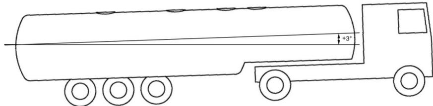
**Figure 46:** Tank truck inclined positively in a longitudinal direction by +3°
