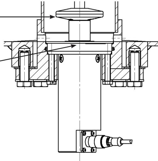
Figure 28: Installation of sensor head, part 2
