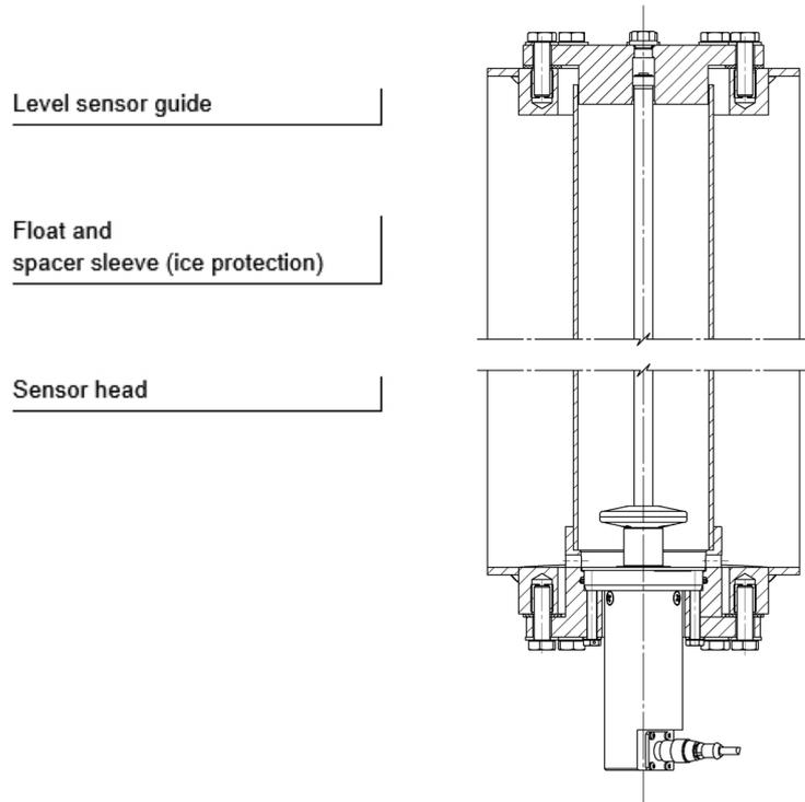
Figure 25: Structure of the sensor head (Drawing 71.251579)
