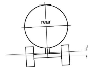
**Figure 48:** Tank truck inclined positively in a transverse direction by +3,0°
