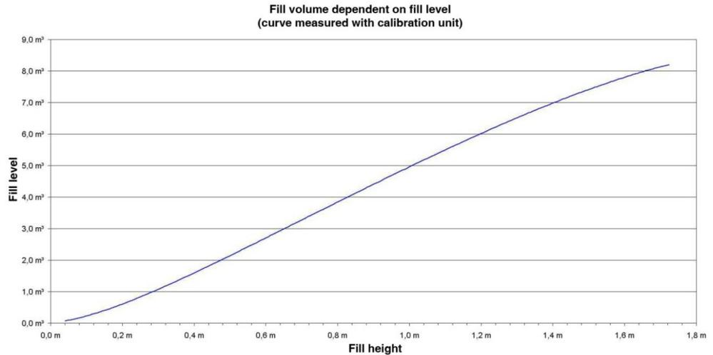
**Figure 5:** Typical fill height – gauge curve
