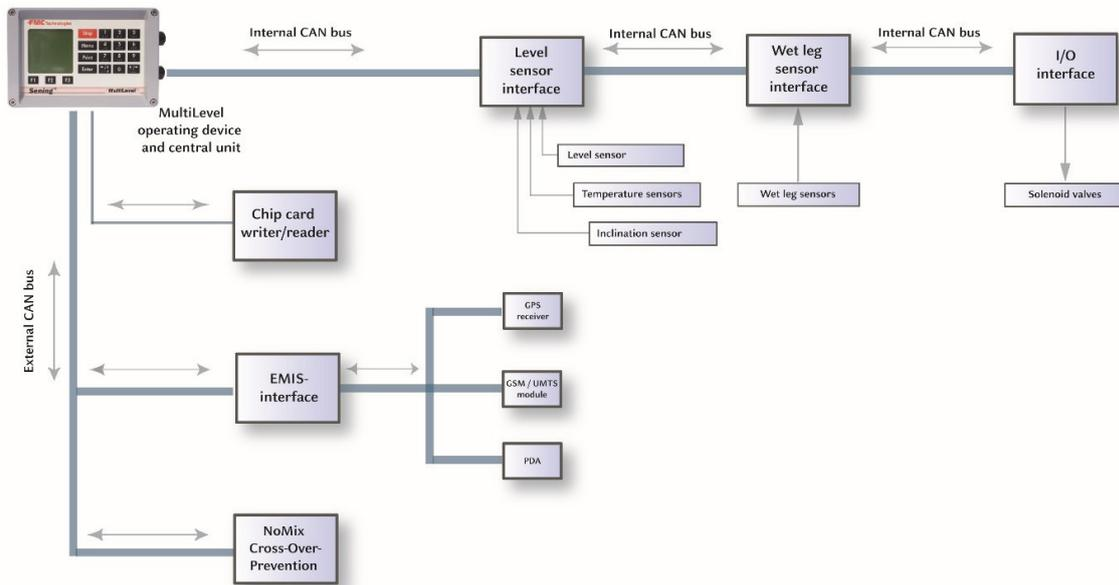
Figure 1: Electrical components
