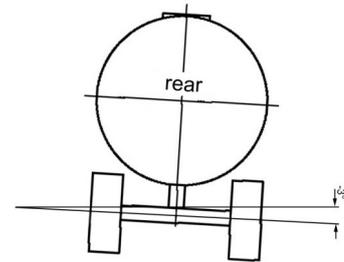
**Figure 47:** Tank truck inclined negatively in a transverse direction by -3,0°
