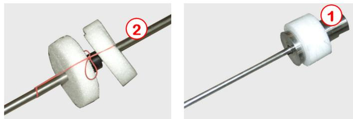
Figure 20: Fixing the foam parts
