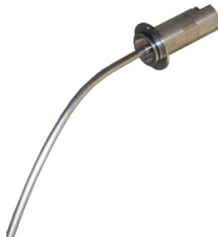
Figure 24: Result of incorrect transport
