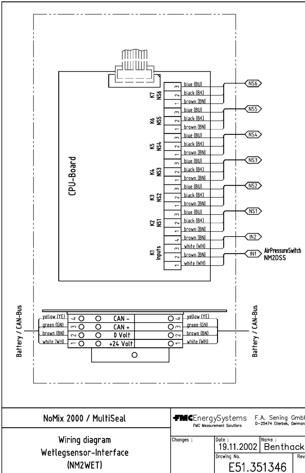
17.1.18. 51.351997 – ML-Wet leg sensor interface, complete – NMN2WET-E
