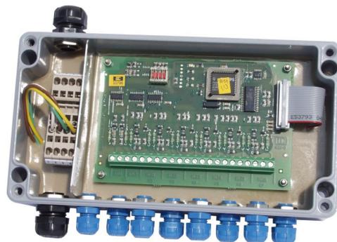
Figure 35: Wet Leg Sensor Interface – NM2WET-E
