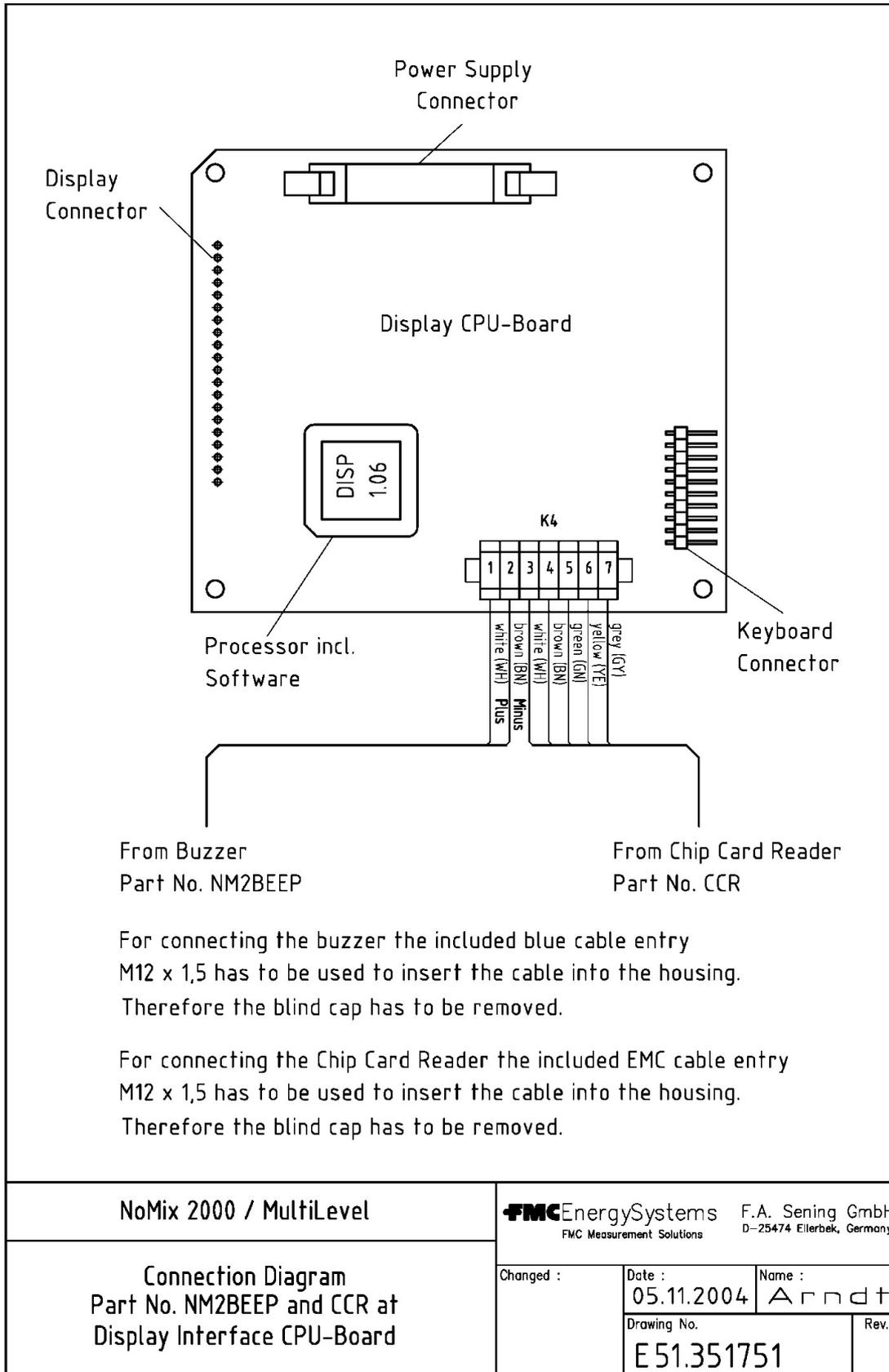
11.351906 – Overall wiring diagram NoMix2000 & MultiLevel – 2 of 2
