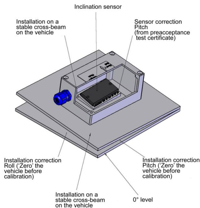
Figure 17: Inclination sensor (drawing: 51.251917)
