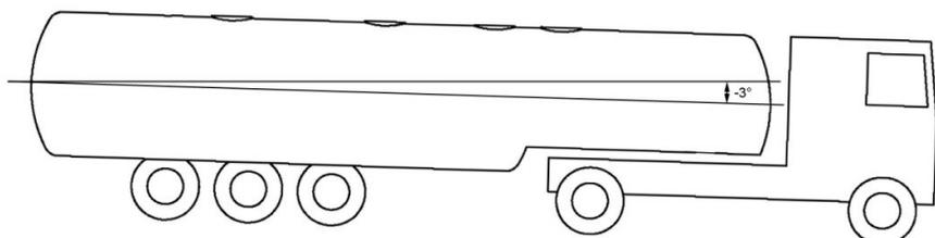
**Figure 45:** Tank truck inclined negatively in a longitudinal direction by -3,0°
