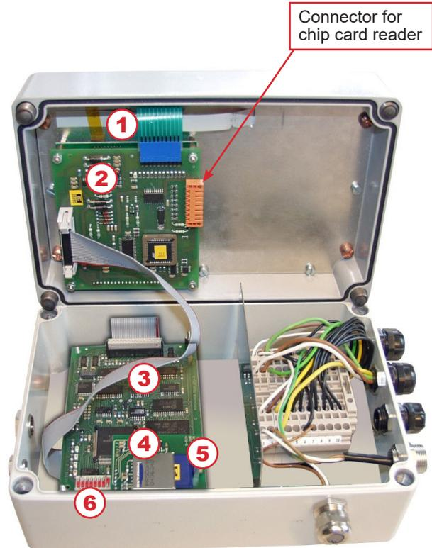
Figure 33: Display Interface 2 / open - with SD-card
