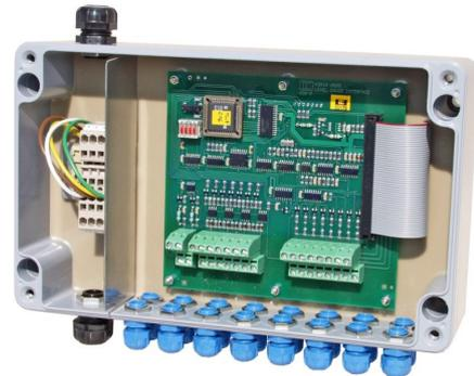
**Figure 38:** Level sensor interface – MLIF
