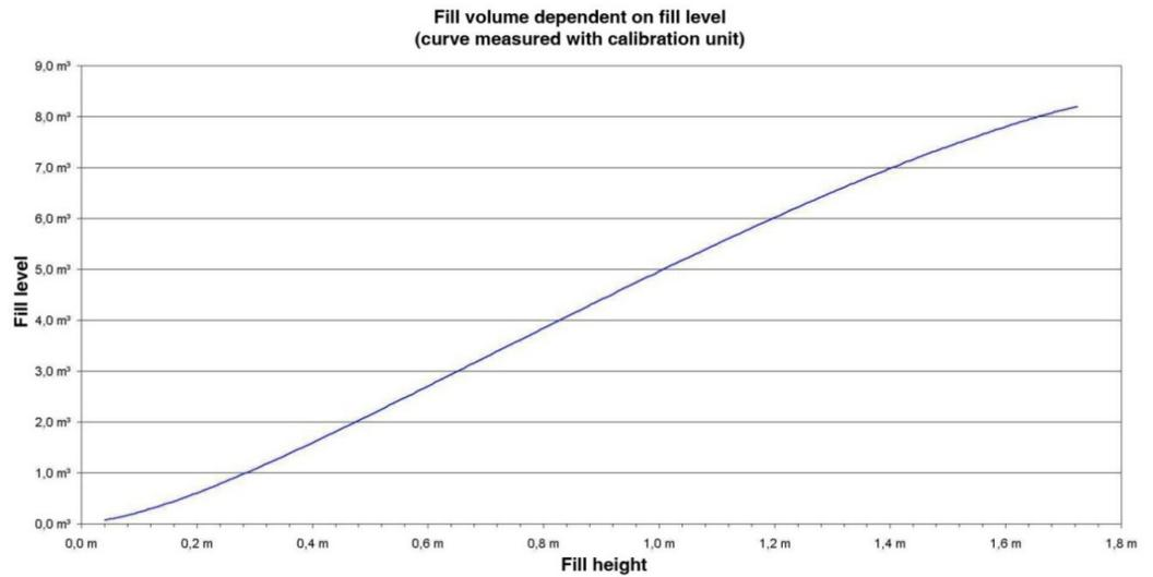
**Figure 13:** Graph of a typical volumetric measurement curve
