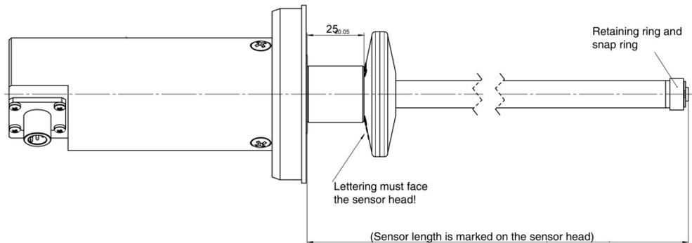
Figure 26: Sensor length (Drawing 25531.351851)
