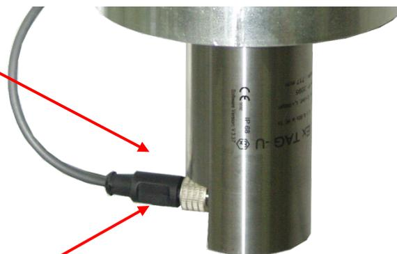
Figure 18: Dipstick plug connection
