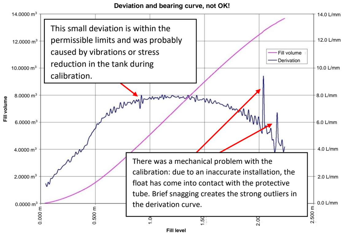
Figure 52: derivation of a bad calibration curve
