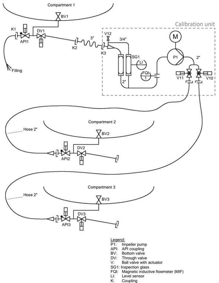
Figure 4: flow diagram of the calibration unit
