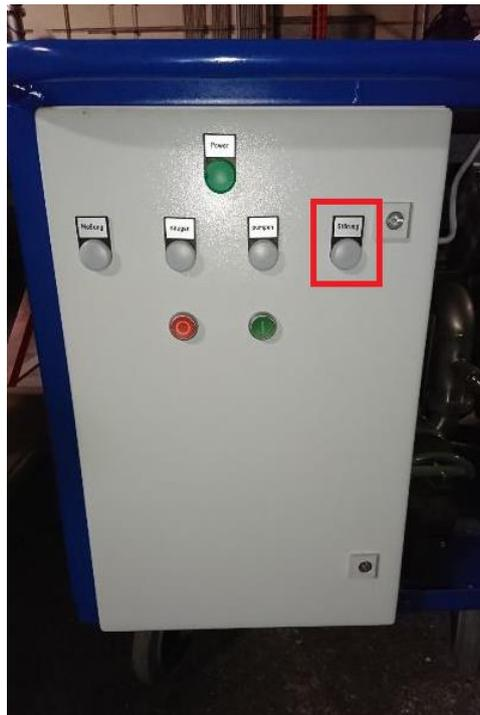
Figure 18: front panel - "Fault" lamp
