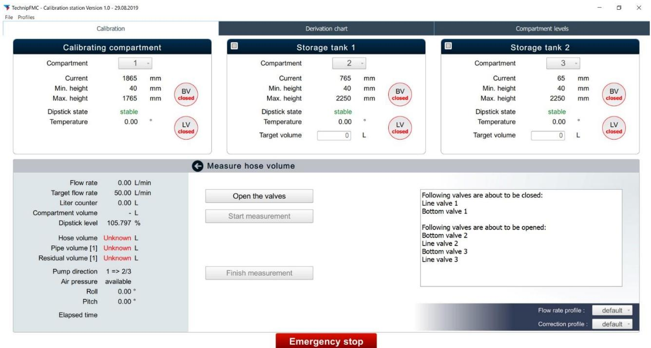
Figure 41: measuring the hose volume
