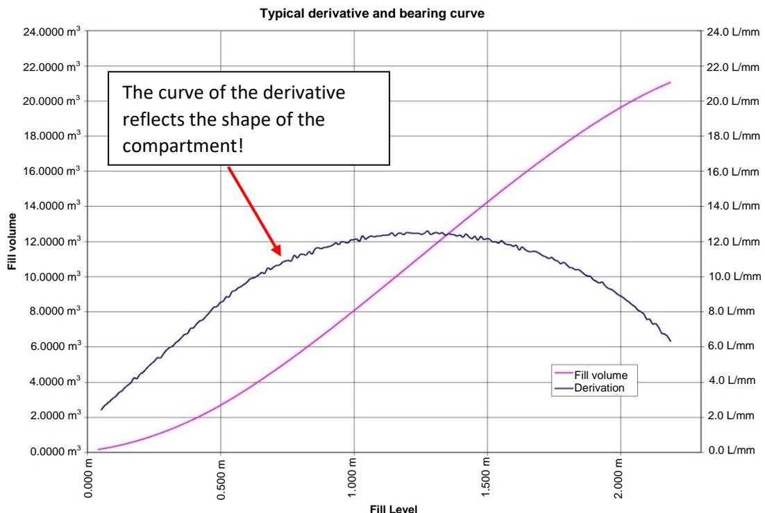
Figure 51: derivation of a good calibration curve
