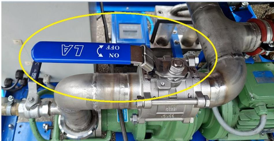
Figure 45: Optional backflow lock – OPEN position
