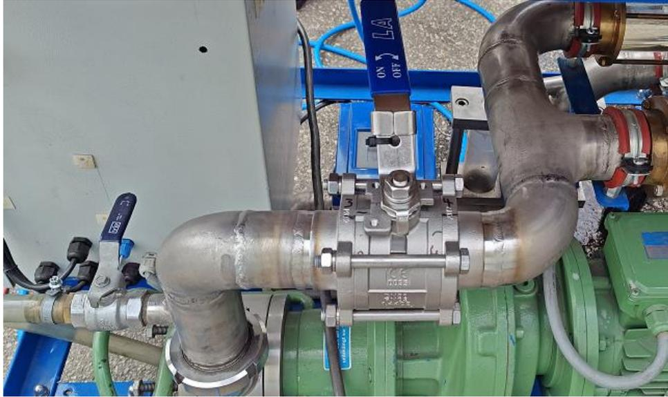
Figure 46: Optional backflow lock – CLOSED position
