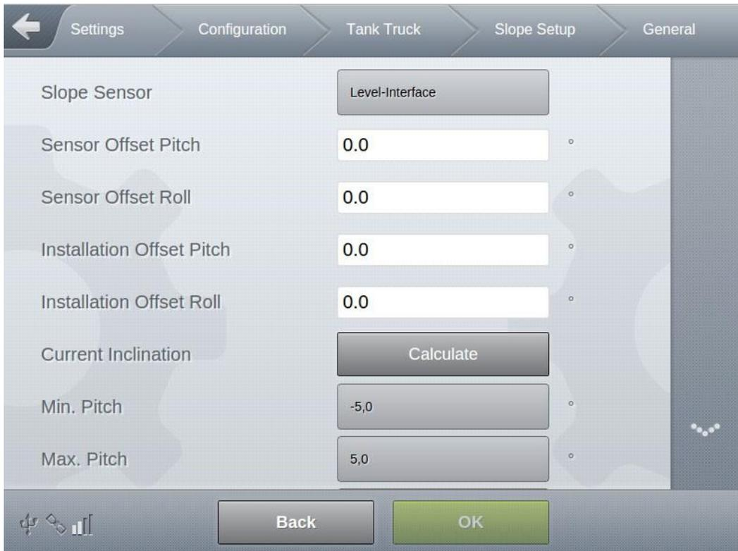
Figure 14: vehicle tilt settings
