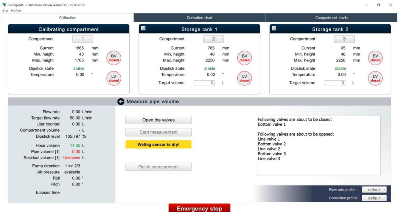
Figure 42: measuring the pipe volume
