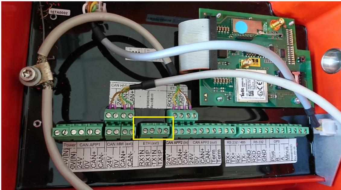
Figure 9: calibration unit Ethernet connection
