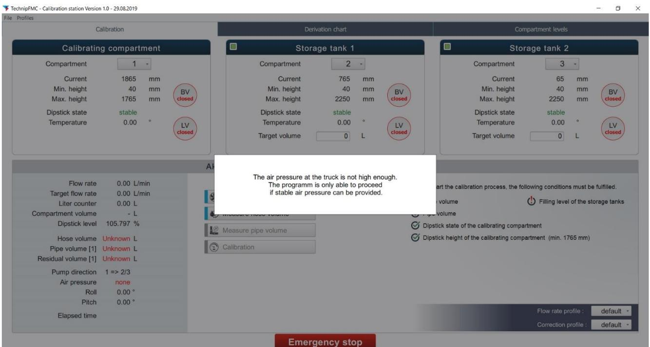
Figure 21: insufficient air pressure
