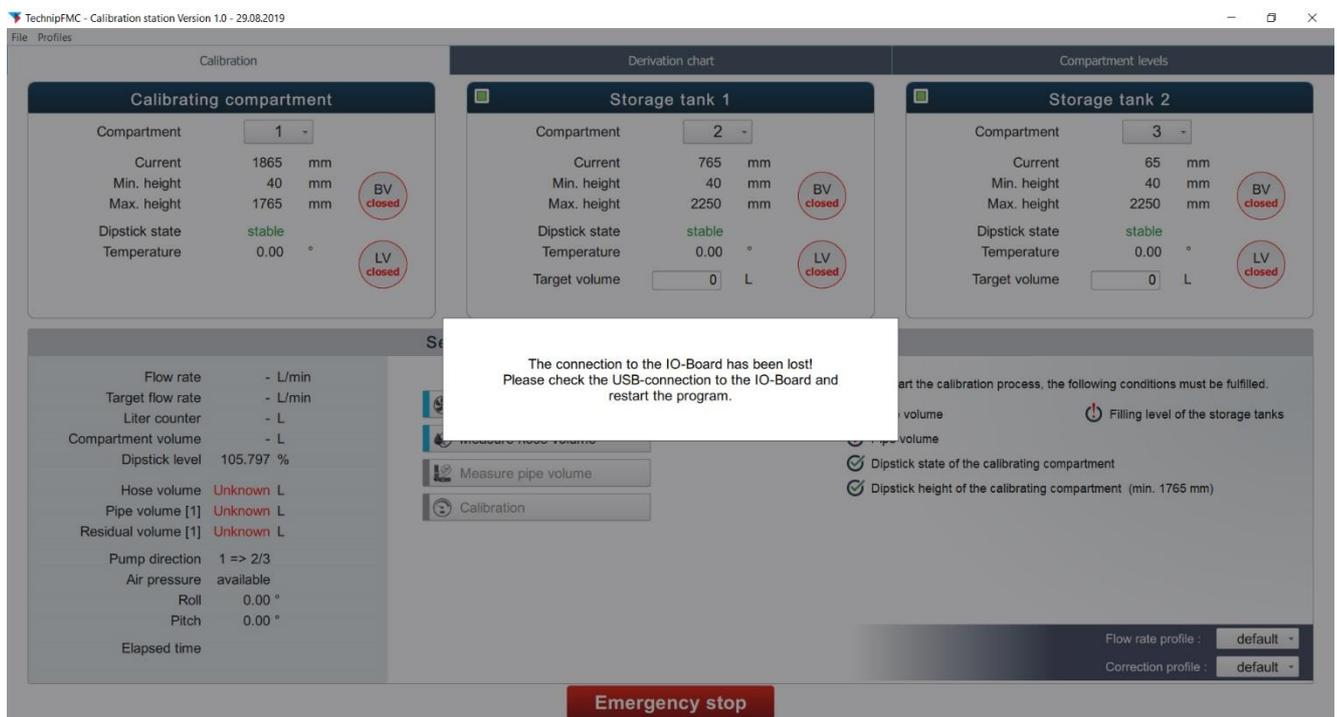
Figure 19: USB connection fault
