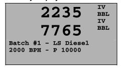
The default delivery display can be replaced with a user configurable display that could display data such as the additive volume, the main product batch size etc.
