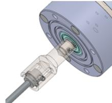
7. Place an o-ring from the adapter assembly into the inside o-ring groove on the underside of the MTC.
