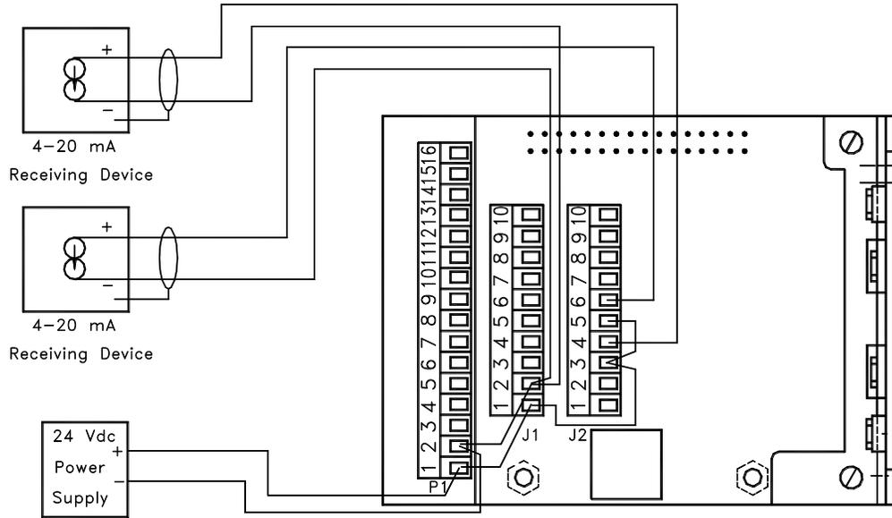
Figure 20. UPCC 4-20 mA Output Wiring
