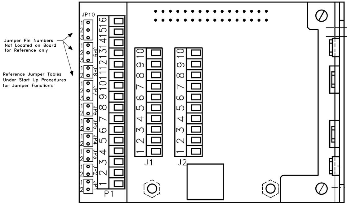
**Figure 5. Jumper Locations (Revision 8 and lower Assemblies)**
