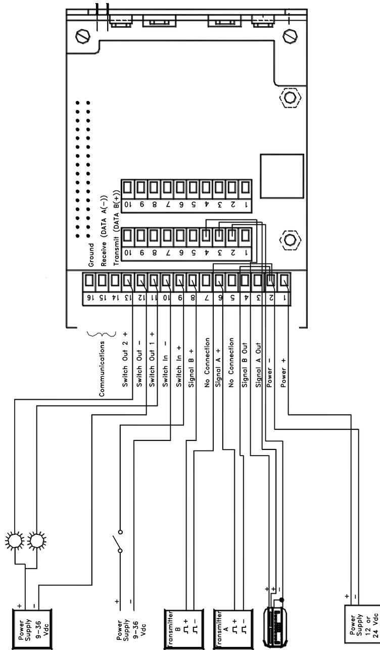
Figure 10. UPCC Typical Wiring with Square Wave Input
