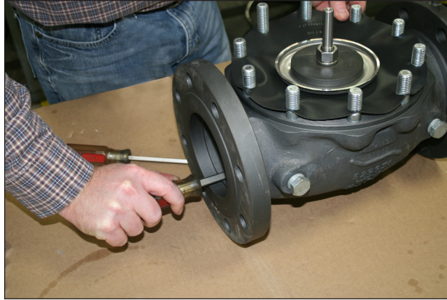
Figure 29 – Stem Assembly Installation
