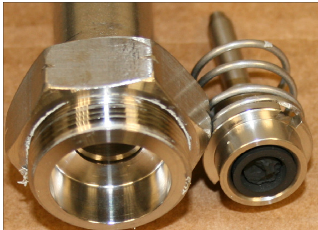
Figure 4 – Solenoid Elastomer Damage Example
