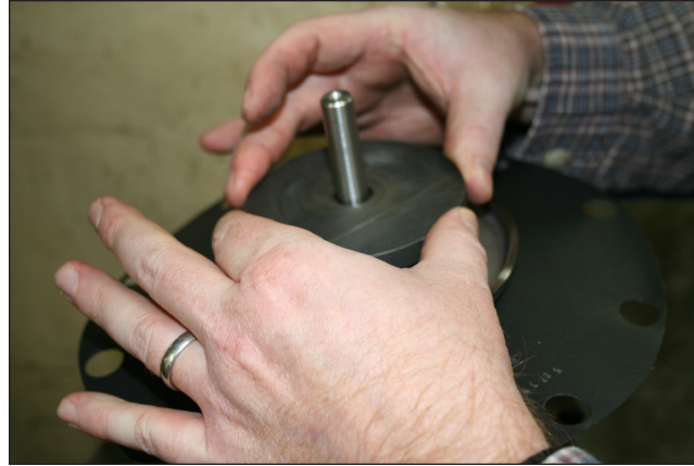
Figure 24 – Back-up Plate Installation
