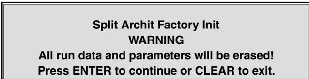
This diagnostic should always be run when a new set of PROMs is installed.
