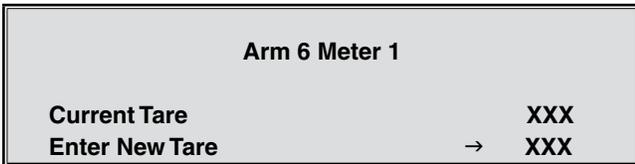
This screen allows the operator to specify a new tare value for a mass meter. Use the keypad to indicate the new tare value and then press ENTER. The display will return to the Mass Meter Diagnostics menu.
