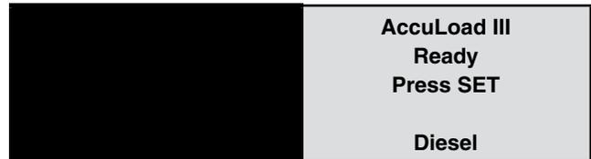
The following screens are displayed if the operator continues the presetting sequence in the split screen view. Note that the amount of information displayed is reduced in this mode, and that many abbreviations are required. Should the operator need more information, he may press the “F2” key to switch to full screen mode, then press “F2” again to revert to the split screen view.
