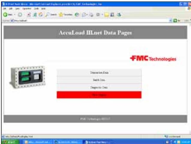
As shown above, the main page has a few options to choose from such as Transaction Data, Batch Data, Diagnostic Data, and Flow Display. The Transaction Data page shows transaction totals, the Batch data page shows batch totals. The diagnostics data shows current hardware configuration or I/O status. The flow display can display a real time view of the current flow on any arm. This display resembles the actual AccuLoad display and is sometimes referred to as a remote flow display.
