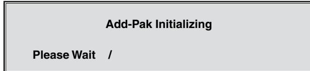
This command will initialize all twenty Add-Pak injectors and reset all parameters and totals back to zero. The AccuLoad will not initialize the Add-Pak injectors as part of its own initialization. When the initialization is complete, the display will return to the Add-Pak Diagnostics menu. Press “CLEAR” to force an early exit out of the display; however, be aware that the Add-Pak may cause an Additive Communications (AC) alarm as it completes the initializing process.
