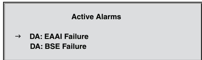
The active alarms can be cleared from this display by moving the arrow to the alarm and pressing “ENTER.” The AccuLoad will then ask for the passcode. When the passcode is entered, the alarm will clear.
