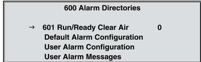
5. Choose the required set of parameters by moving through the menu using the up and down arrow keys on the keypad.
