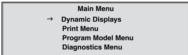
2. Move the arrow to the Program Mode menu and press "ENTER." This will display the "Enter Passcode" screen.
