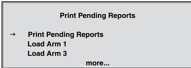
Once the selection is made, the AccuLoad will display the # of pending reports to be printed.
