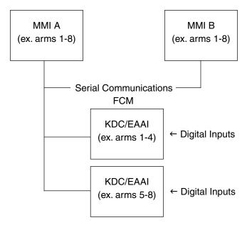
Digital inputs on each KDC/EAAI board set are used to identify the current position of the load arm. The two MMIs are connected to the same communications port on each KDC, and take turns polling for an arm that is positioned for it. MMI Configuration Parameter 002 is used to indicate whether an MMI is a standalone unit, or if the MMI should be labeled "A" or "B".
