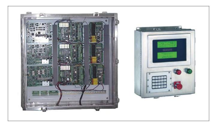
The AccuLoad III-SA consists of a cabinet housing up to four board sets, and a remote Man Machine Interface (MMI). The MMI is the device from which the board sets are configured and controlled. The cabinet and boards are shown above on the left, and the MMI is shown on the right. The MMI controls up to 18 load arms, with a maximum of six transactions in progress at any given time. Any load arm configuration currently supported by AccuLoad III-X firmware is available using this system.
