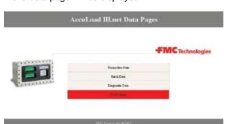
As shown above, the main page has a few options to choose from such as Transaction Data, Batch Data, Diagnostic Data, and a Flow Display. The Transaction Data page shows transaction totals, the Batch data page shows batch totals. The diagnostic data shows current hardware configuration or I/O status. The flow display can display a real time view of the current flow on any arm. This display resembles the actual AccuLoad display and is sometimes referred to as a remote flow display.
