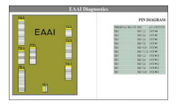
The EAAI also has the ability to display its current status. In the below example, the Raw A/D Count, the Raw Analog Value, and the Engineering Value is shown. Any input or output has the ability to display its status, value, or state that it is currently in.
