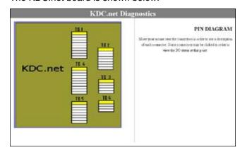
This shows the KDC.net board with an example of the mouse over function. The corresponding pin connection information is for the Com 1 connector (TB1).
