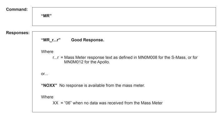
**Remarks:** See "MC" for a description of how to send a command to the mass meter.
