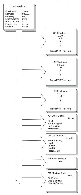
The IP, Netmask and Gateway Addresses are in the form of four numbers separated by ".". The range of each number (also known as "octet"), is 0-255. The microLoad.net screen for entering these values lists the present octet values vertically.
