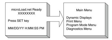
Select "Program Mode Menu" and depress the ENTER key. The microLoad.net will then request the passcode to allow entry into Program Mode Menu. The default passcode for a new microLoad.net is "0000". After entering the proper passcode the Program Mode Menu screens will be accessible.
