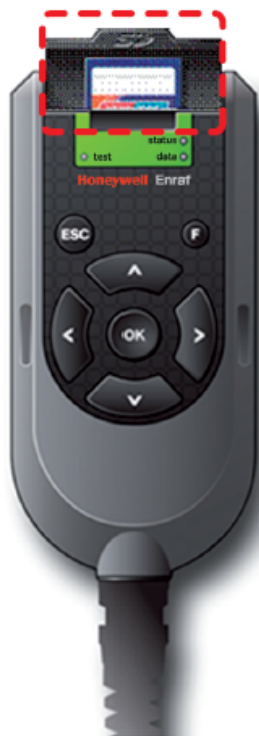
Figure 5-4: SD card location in the LAD (lid opened)
