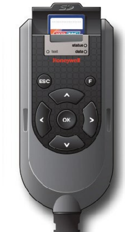
Figure 5-5: SD card location in LAD (lid opened)
