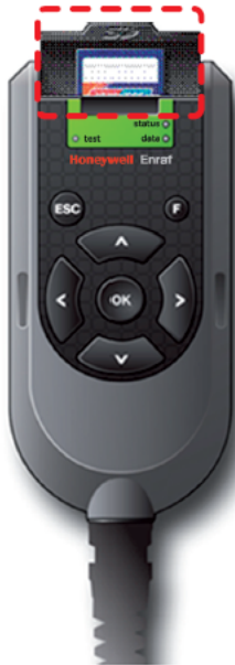
Figure 4-3: SD card location in LAD (lid opened)
