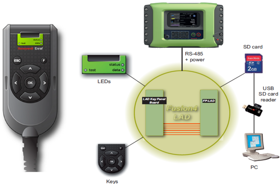
Figure 4-1: LAD and its system overview
