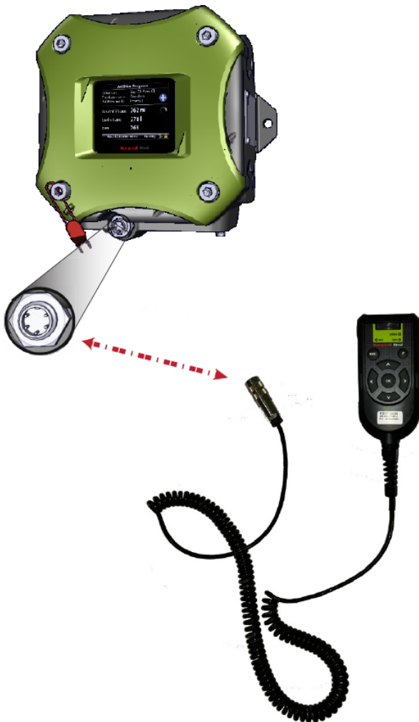
Figure 3-1: Connecting a LAD to the SSC-A / SSC-B device
