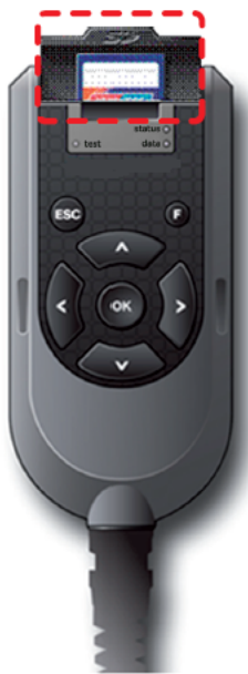
Figure 4-3: SD Card Location in LAD (lid opened)
