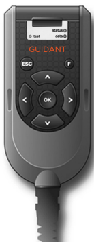
Figure 2-1: Local Access Device (LAD)
