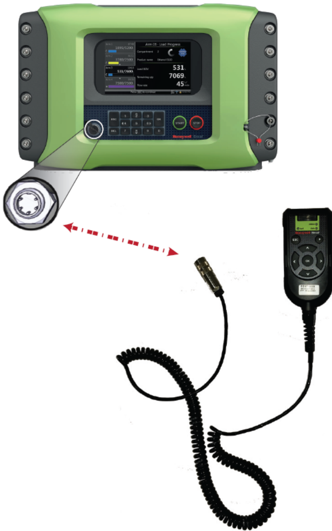
Figure 3-2: Connecting a LAD to the MSC-A / MSC-L device
