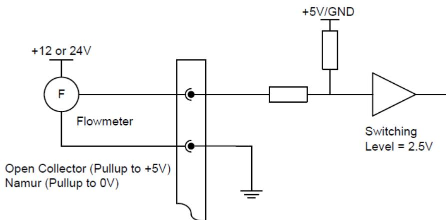
The type of flow meter input can be selected through the configuration menu.
