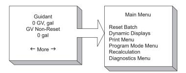
Select "Program Mode Menu" and depress the ENTER key. The microFlow.net will then request the pass-code to allow entry into Program Mode Menu. The default pass-code for a new microFlow.net is "0000". After entering the proper pass-code the Program Mode Menu screens will be accessible.
