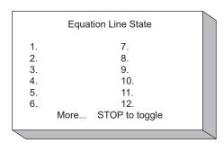
Entering the equation number that is to be disabled and pressing ENTER will change the status on the screen from either T (True) or F (False) to D (Disabled). The equation from that point until enabled will not be active. To enable an equation the same process is followed, except that the screen will indicate that the equation is D (Disabled). Entering the equation number will enable that equation.
