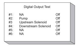
Moving the arrow to the output that is to be tested and pressing ENTER will change the state of the output. An example would be moving the arrow to output #2 Pump and pressing ENTER.
