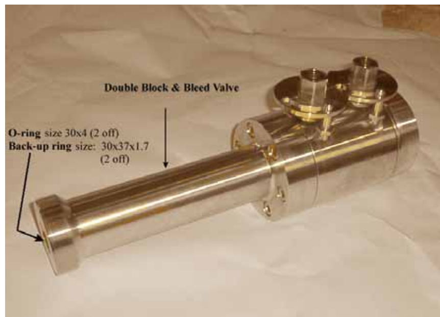
Picture 6. Double Block & Bleed Valve
