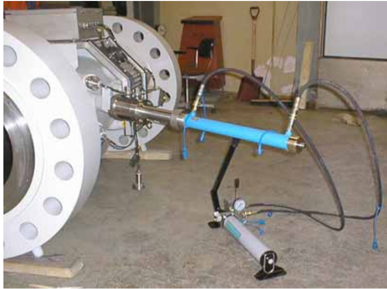
Picture 11. Complete TRT mounted on the MPU
