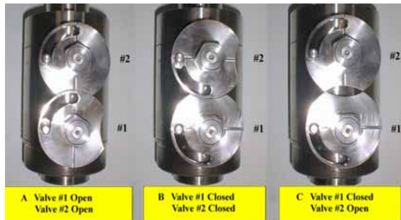
Picture 10. Double Block & Bleed Valve, Open/Close positions
