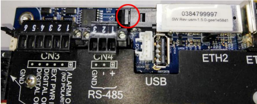
**WARNING:** To remove blank protective plug press down on tab and slide back. Do not remove protective plug until ready to insert fiber cable assembly terminated with mechanical transfer registered jack (MT-RJ) connector to prevent contamination of the optic components.
