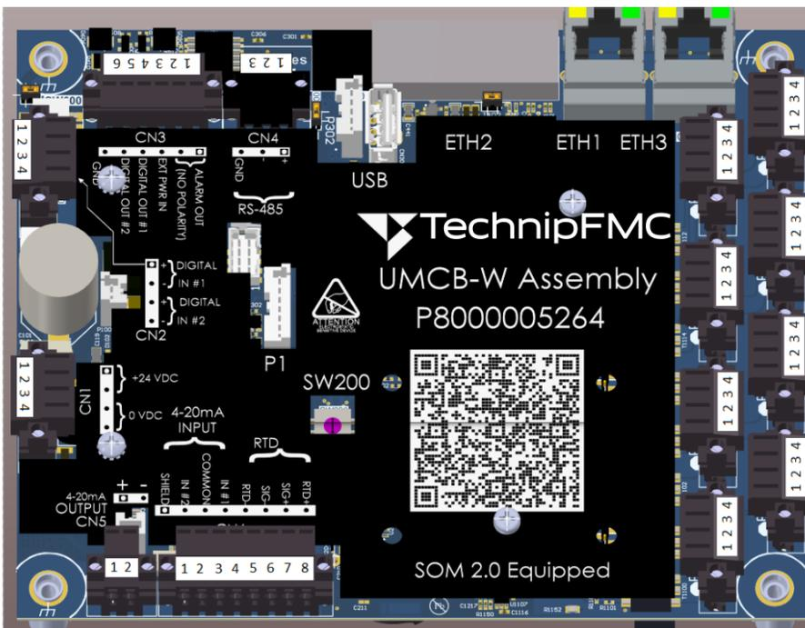
**NOTE:** UMCB board, Revision A and above, equipped with second generation system on module (SoM), Revision A legend shown.
