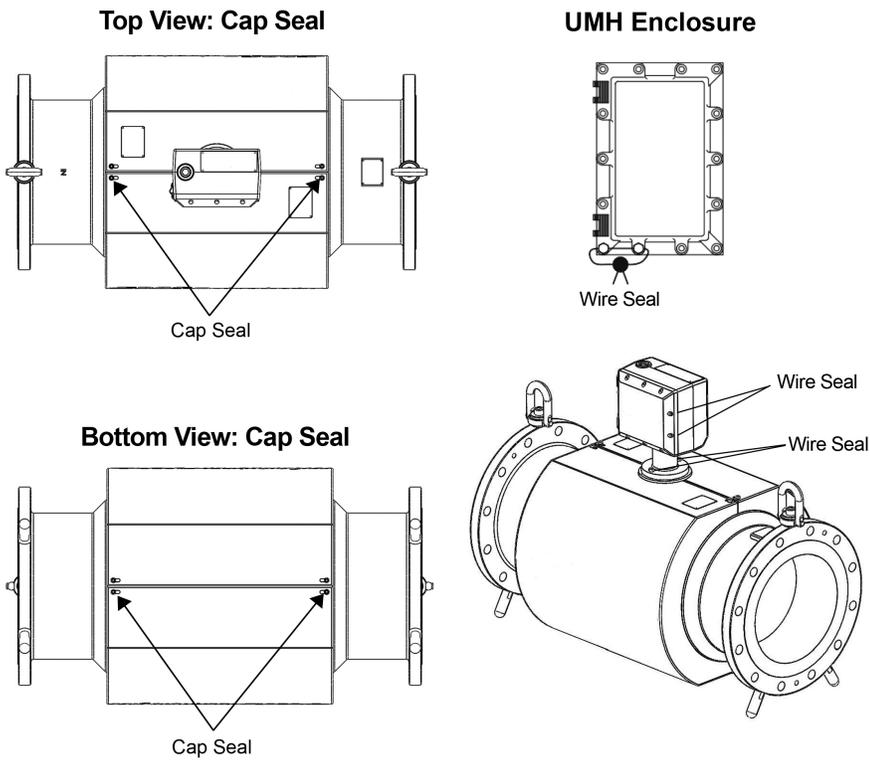
Figure 102: Enclosure Sealing
