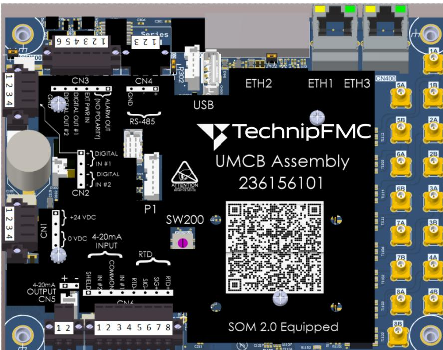
**NOTE:** UMCB board, Revision C and above, equipped with second generation system on module (SoM), Revision C legend shown.
