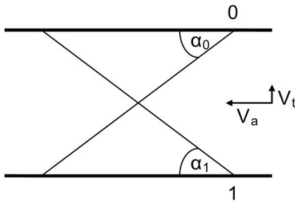
By checking the direction and magnitude of the transverse flow components in the two upper planes, the flow regime can be determined, as shown in the following picture:
