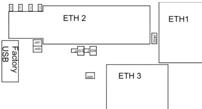
Figure 27: Bottom View of UMCB Board Revision 3 or Older
