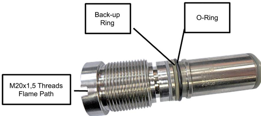
O-rings facing the natural gas are made of Fluoroelastomers (FKM). The O-ring manufacturers do not specify any exact lifetime of the O-rings, but during normal operation (continuously pressurized and untouched) the O-rings will last for several years. However, to be on the safe side it is strongly advised to:
