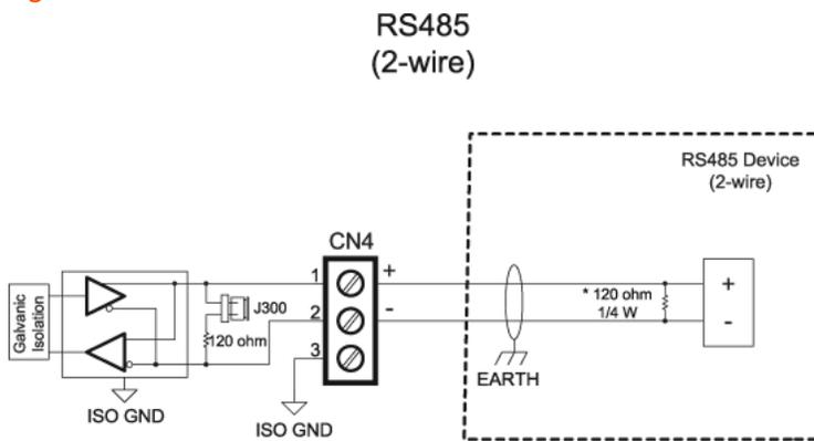
**NOTE:** Customer-supplied resistor is only necessary if customer equipment does not have internal termination.
