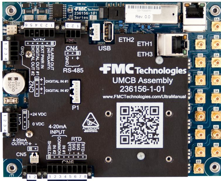
**NOTE:** On the UMCB cover shield legends connector position 1 is indicated by a circle enclosed in a square.
