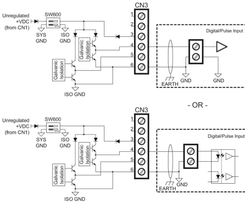
**NOTE:** \*Out2B is wired identically between position 5 and 6.
