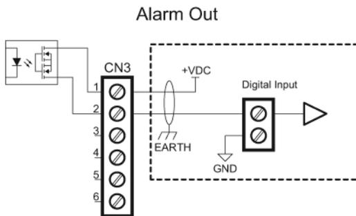
The solid state relay (SSR) is closed during normal operation. During an alarm, or when the power is off the SSR is open. The relay is direct current (DC) only.
