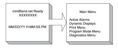
Select "Program Mode Menu" and depress the ENTER key. The miniBlend.net will then request the passcode to allow entry into Program Mode Menu. The default passcode for a new miniBlend.net is "0000". After entering the proper passcode the Program Mode Menu screens will be accessible.
