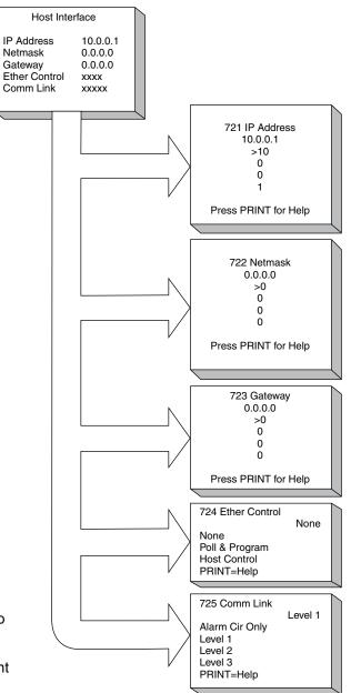
The IP, Netmask and Gateway Addresses are in the form of four numbers separated by ".". The range of each number (also known as "octet"), is 0-255. The miniBlend.net screen for entering these values lists the present octet values vertically.
