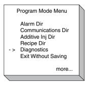
Pressing ENTER with the arrow in front of Diagnostics will display six items of the Diagnostics Menu. Pressing the up and/or down arrows will step through the Diagnostics Menu. The available diagnostics in the order that they appear on the menu are as follows:
