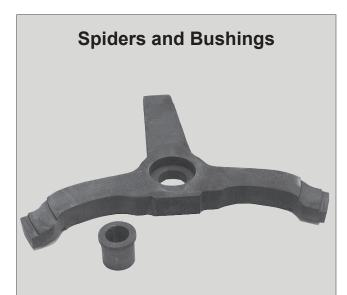
Locates rotor assembly while obtaining blade tip and block clearances on rotary vane PD meters. Tightens rotor (gear set) without the cover and allows visual inspection of clearances on oval gear meters.
