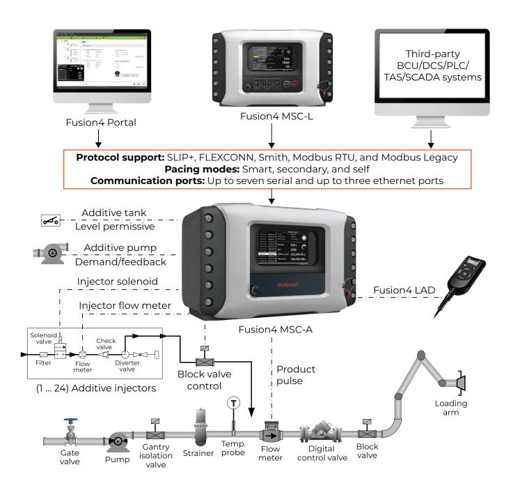
Graphic representation showing a basic setup of the additive controller. Additional interfaces might be needed based on site requirements.
