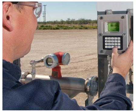
The microFlow.net Liquid, shown interfacing with a Coriolis meter, is designed for flow management to monitor, temperature compensate, and transmit data to a data collection system.
