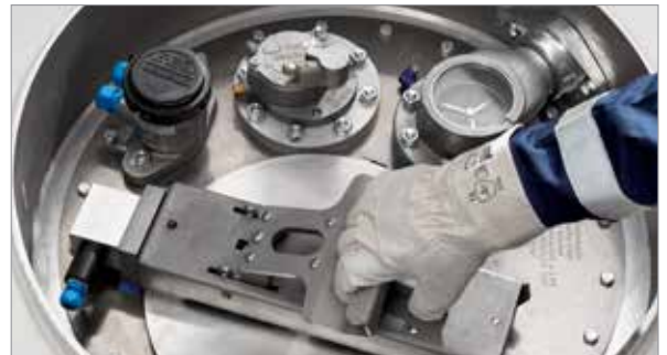
Manlid with flame arrestor DBG2-2 combined with vent valve DO702-F, pneumatic sensor HANV and electrical overfill prevention NSE A6-2.
