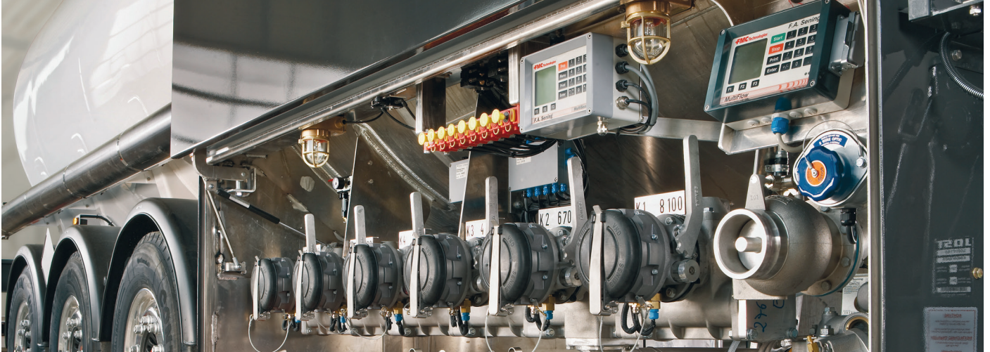
MultiFlow with GMVZ1004 meter gas extractor package in combination with MultiSeal (SPD) on a service station delivery truck in Bulgaria
