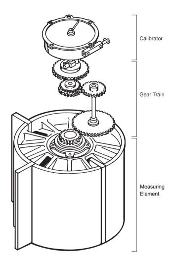
Six threads exposed on the adjustment screw is a good starting point to begin calibration with new calibrators and a 96% geared meter. On meters with Automatic Temperature Compensation, each notch provides a change equal to the Coefficient of Expansion per degree F. For example, an ATC calibrator for 38° API would provide .00046 per notch as 38° API has a Coefficient of Expansion of .00046/°F.
