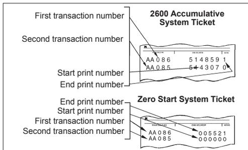
**2600 Accumulative System Ticket** – Delivery output is obtained by subtracting Start Print from Finish Print.
