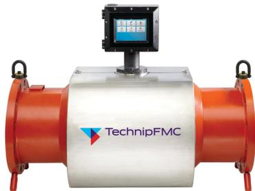
The Smith Meter® Ultra 4c liquid flowmeter is a four-path ultrasonic meter for custody transfer measurement of petroleum products. The meter provides highly accurate measurement over a range of light to medium crude oils and refined products using an exclusive four-path design.
