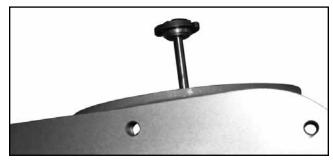
Step 2. Remove the output shaft.
