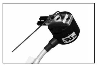
**Step 5.** Disassemble the torque arm assembly from the encoder by removing the two outer screws then the two inner screws.
