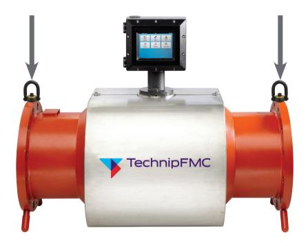
Do not lift or move the meter by placing any device through the center bore of the meter or around the meter mounted electronics enclosure. Also take caution with any lifting straps or cables that they do not touch or place any pressure on the meter mounted electronics enclosure.
